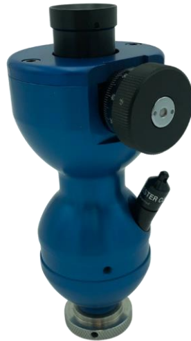
King 100 Brinell scope 20x 0.01mm resolution
